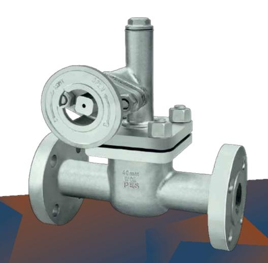
PES Cast Steel Parallel Slide Blow Down Valve, Rack & Pinion operated with renewable stainless steel trim, Flanged ends, Flanges as per ASME B16.5 Class-300. Maximum service temp. 400°C. Each Valve is supplied with operating key.
